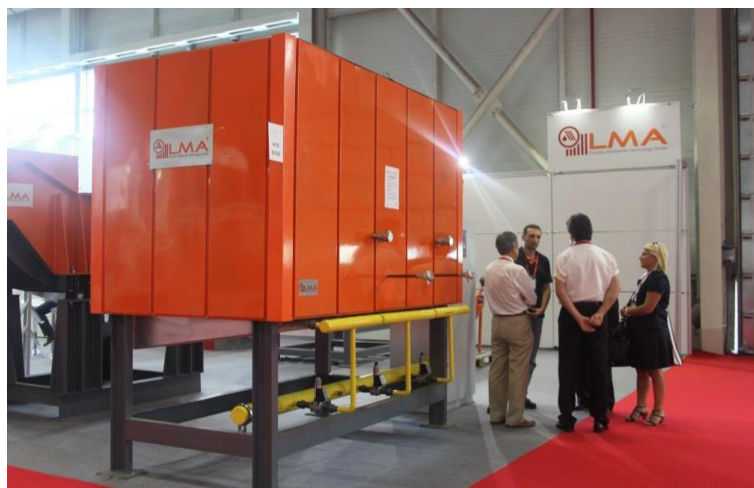
Figure-13: Thermal reclamation system
