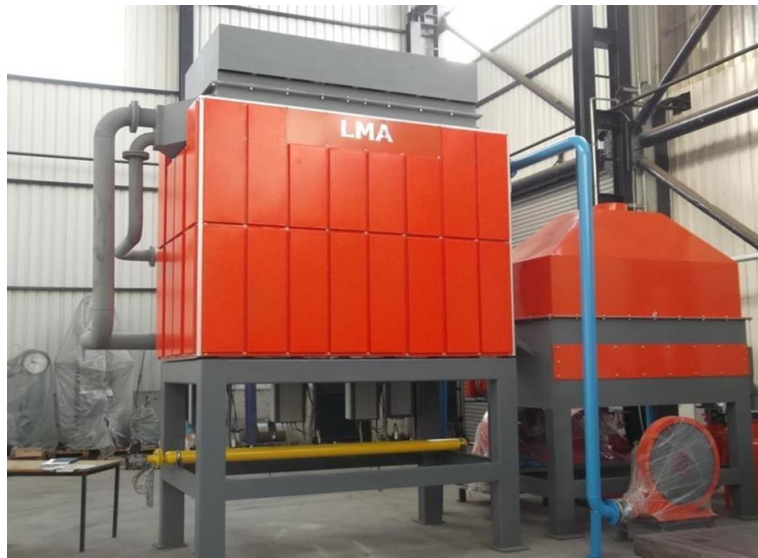
Figure 14:LMA Thermal reclamation systems
